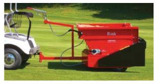
The Rink TB950 is a wheel driven topdresser and can be pulled by virtually any vehicle. The brush and conveyor belt are driven by the 4 wheels (or optional by 2 wheels), ensuring a consistant application rate.
