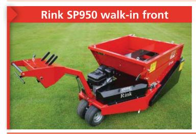
The Rink SP950 contains a 6,5hp engine, and the weight of the machine is evenly distributed over 6 wheels in order to minimize ground pressure.
