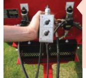
Optional: an electrical control panel, carried to the operator seat, controls the belt and spinner speed
