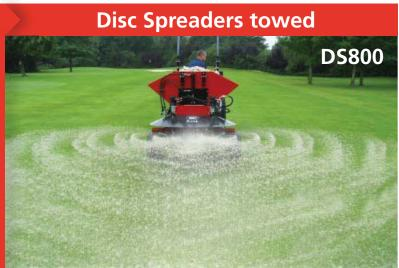
These disc spreaders have a hopper capacity of 0.55m<sup>3</sup>, 0.8m<sup>3</sup> and 1.2m<sup>3</sup> (level). The operation of the belt and spinners is done from the tractor seat.
